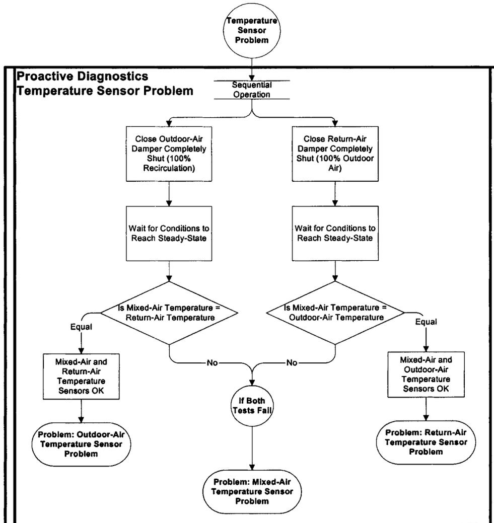
Fig. 5 Decision tree to isolate the faulty temperature sensor
