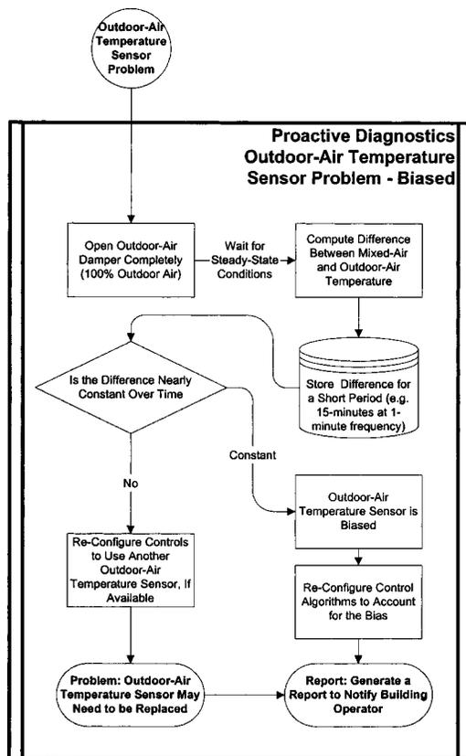
Fig. 6 Decision tree to check if the outdoor-air temperature sensor is biased and implement a temporary correction
