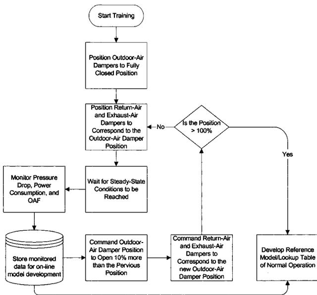
Fig. 8 Overview of the process to develop a reference model to characterize the normal operation of an outdoor-air damper
