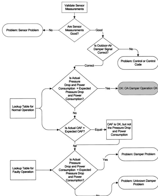
**Fig. 11 Decision tree to detect and diagnose outdoor-air damper faults**
