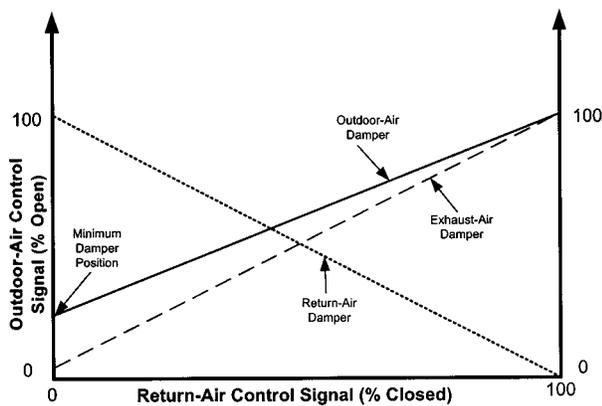
Fig. 9 Relationship of the damper positions during normal operations
