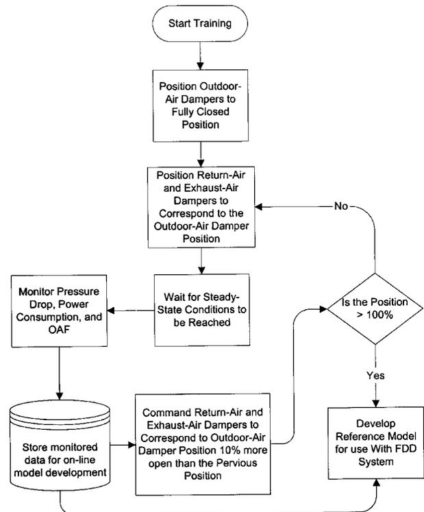
Fig. 10 Overview of the process to develop a reference model to characterize the outdoor-air damper stuck fully closed
