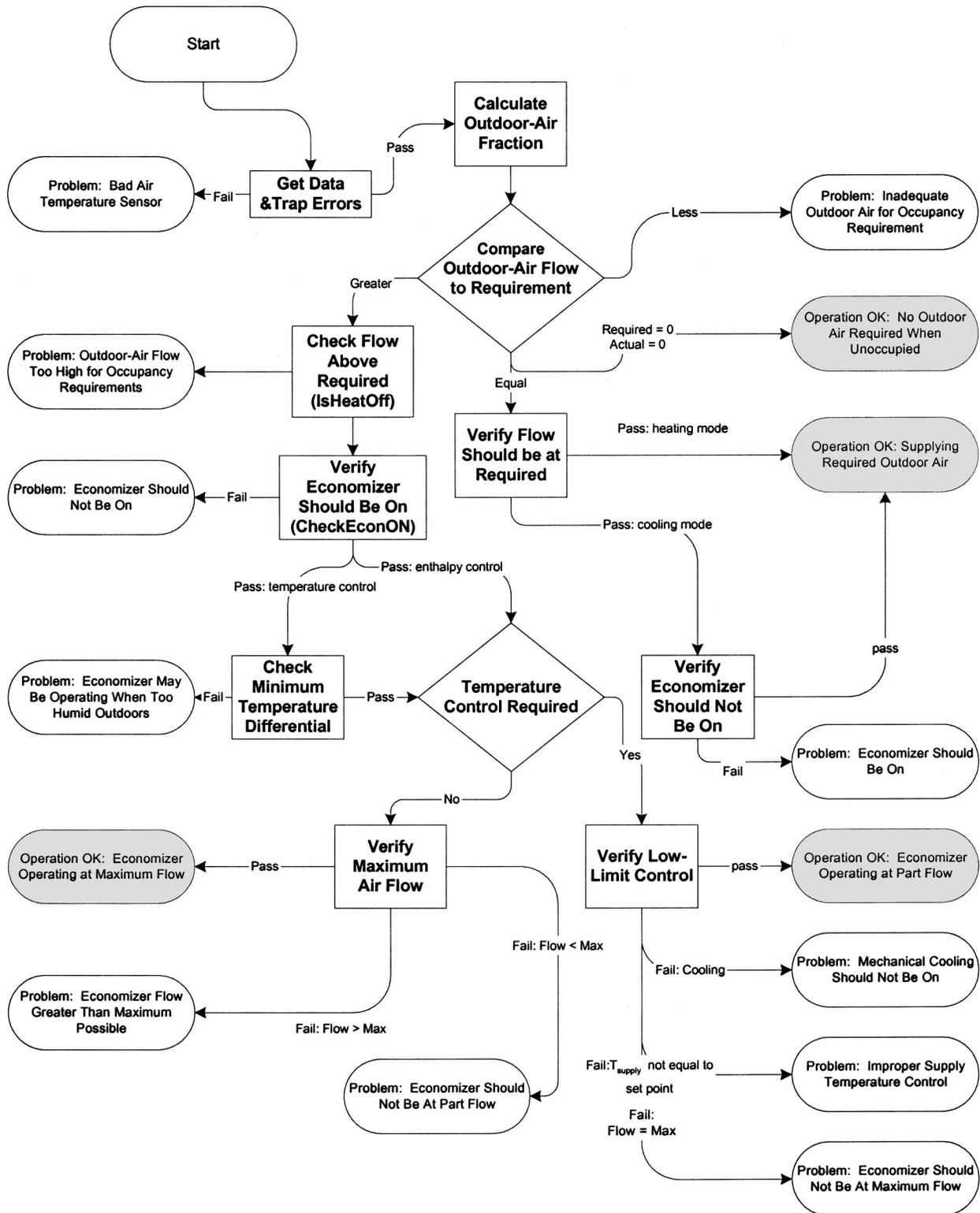
Fig. 4 Overview of the passive part of the automated proactive commissioning process for an AHU (including economizer and ventilation operations)
