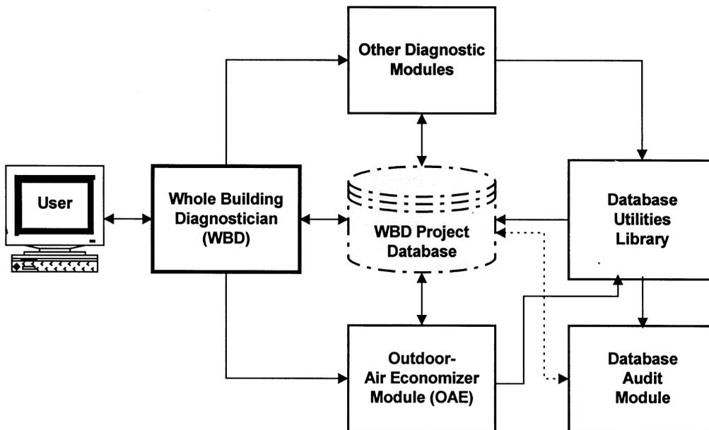
Figure 2 Whole building diagnostician—software architecture.
