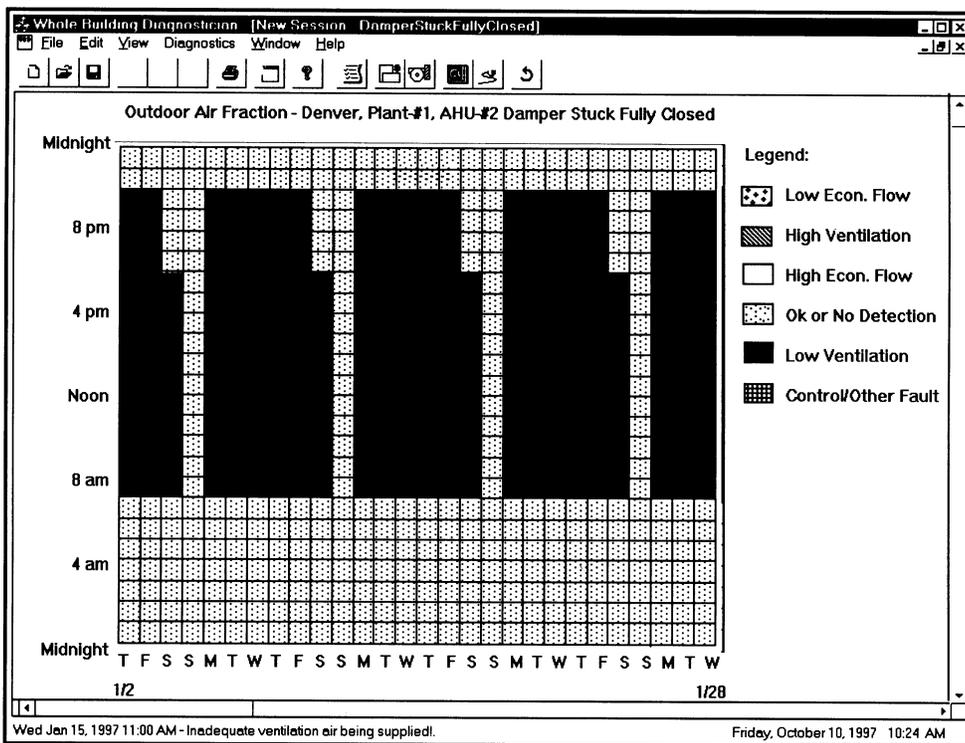
**Figure 6** Diagnostic results showing proper (small dot patterns) and faulty operation (patterns) for a data set with an outdoor-air damper stuck fully closed.
