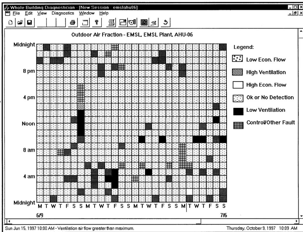
Figure 9 Diagnostic results for AHU-06 at the EMSL building.
