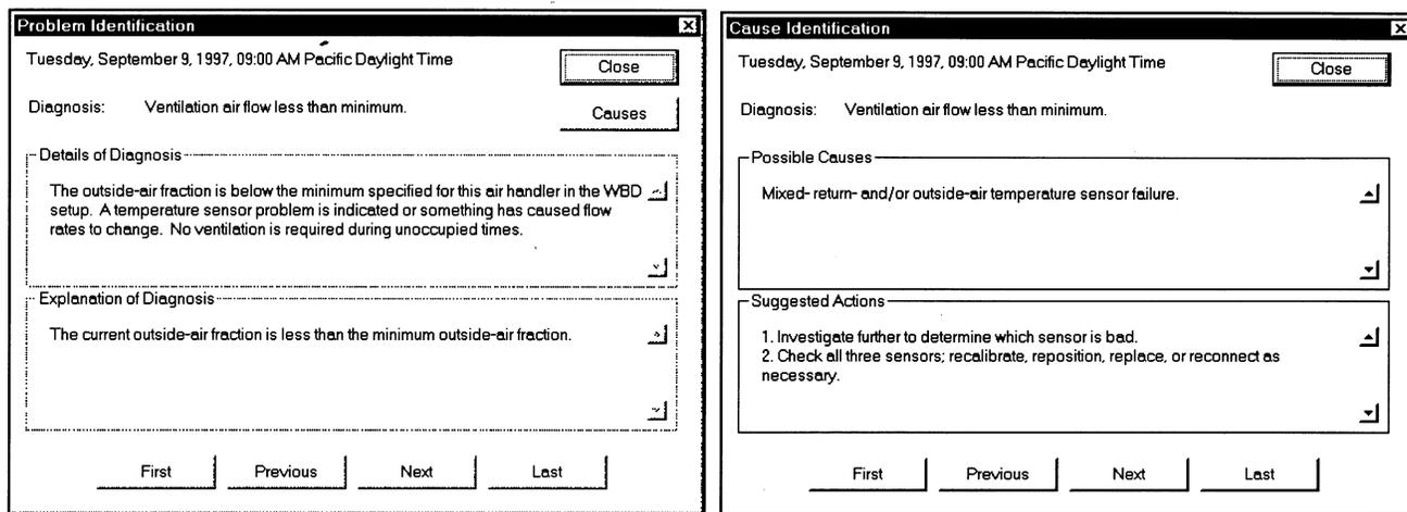
Figure 5 Screen on the left shows the details of the diagnosis and a description of how the diagnosis was obtained; the screen on the right shows a possible cause for the problem identified and suggested actions to correct the problem.
