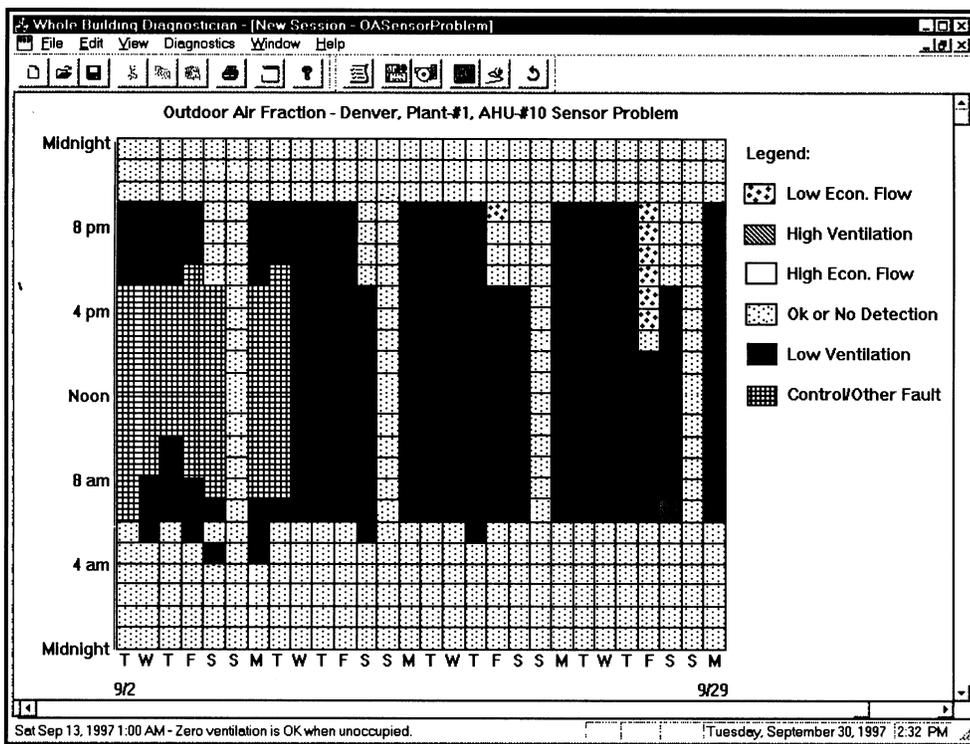
Figure 4 Diagnostic results showing proper (small dot pattern) and faulty operation (other than the small dot pattern) for a data set having a faulty outdoor-air sensor.
