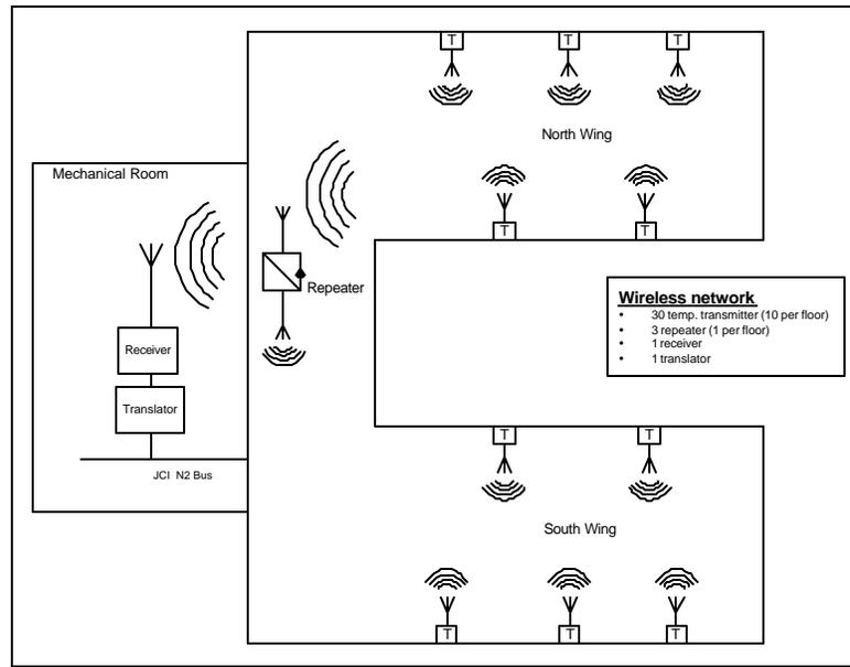
**Figure 1: Layout of Wireless Sensor Network. The building has 3 identical floors. Shown is only one floor.**
